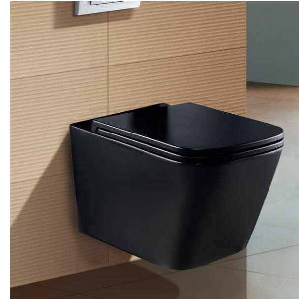
SF 9625-1-BLACK Washdown Wall-hung Closet With UF seat cover Color: Matt Black Size: 510x345x340mm (20.4"x13.8"x13.6") P-trap, 180mm, Roughing-in
