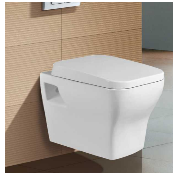
SF 9611 PP COVER Washdown Wall-hung Closet With PP seat cover Color: White Size: 485x355x420mm (19.4"x14.2"x16.8") P-trap, 180mm, Roughing-in
