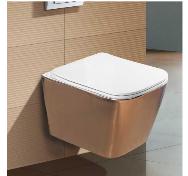
SF 9625-2-RG Washdown Wall-hung Closet With UF seat cover Color: Inner White Outer Rose Gold Size: 510x345x340mm (20.4"x13.8"x13.6") P-trap, 180mm, Roughing-in
