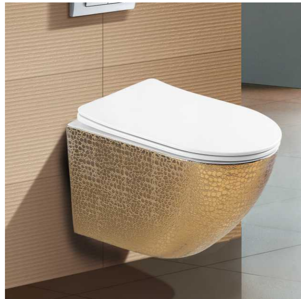
SF 9616-2-G Washdown Wall-hung Closet With UF seat cover Color: Inner White Outer Gold Size: 495x365x360mm (19.8"x14.6"x14.4") P-trap, 180mm, Roughing-in
