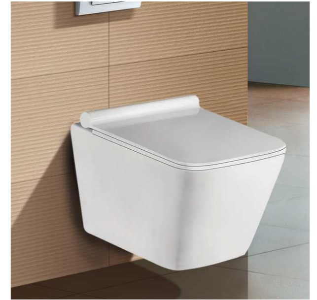
SF 9620 Washdown Wall-hung Closet With UF seat cover Color: White Size: 500x355x415mm (20"x14.2"x16.6") P-trap, 180mm, Roughing-in
