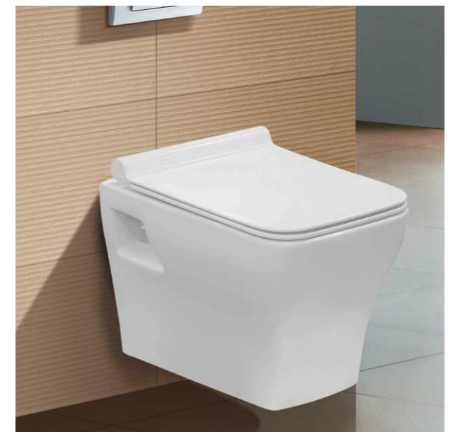
SF 9611 UF COVER Washdown Wall-hung Closet With UF seat cover Color: White Size: 485x355x420mm (19.4"x14.2"x16.8") P-trap, 180mm, Roughing-in
