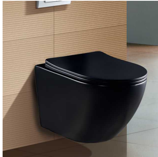
SF 9616-1-BLACK Washdown Wall-hung Closet With UF seat cover Color: Matt Black Size: 495x365x360mm (19.8"x14.6"x14.4") P-trap, 180mm, Roughing-in
